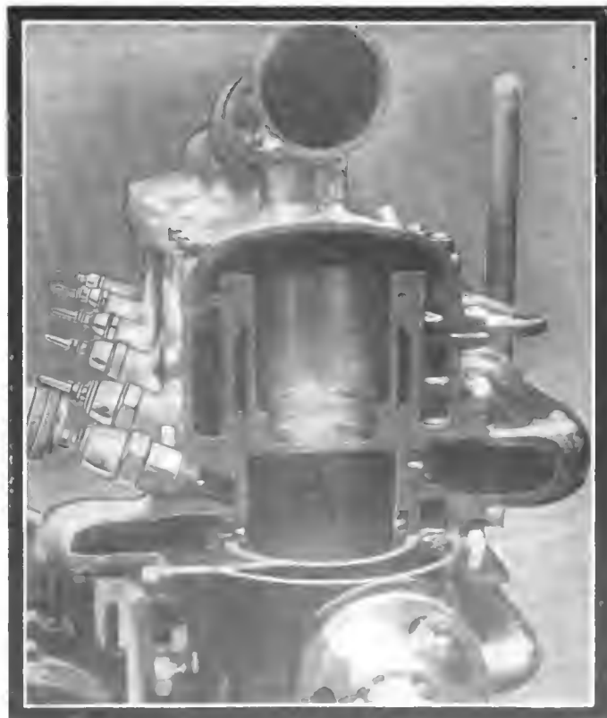
Fig. 11—Section of the Rolland Pilain sleeve-valve motor
